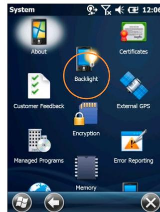
4. Check the **“Turn off the backlight if device not used for”** box and select the preferred length of inactivity before activation of the **screen off** power saving function from the pull-down menu. Shorter *off* delays will increase battery power conservation.
