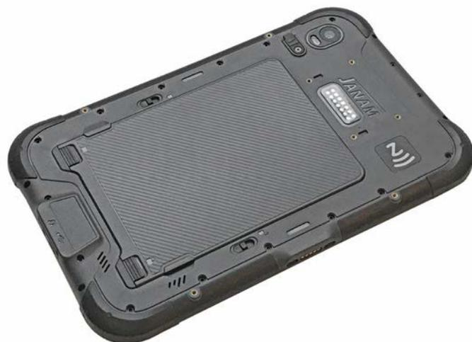
Once all four retaining sliders are in the open position, use a plastic opening tool, a fingernail, or a small coin to carefully pry open and then remove the battery compartment cover. If you use a coin or metallic tool such as a flat blade screwdriver, make sure not to scratch the housing or damage the compartment seal.
