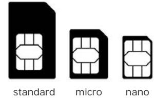
The HT1 SIM card slot is designed for use with a **micro SIM card**. A standard SIM card is too large and will not fit. If a SIM card provided by your cellular carrier uses the nano format, you need a (readily available) micro SIM card adapter to use it in the HT1. Contact Janam or your local wireless carrier for more information about SIM cards and wireless service.
