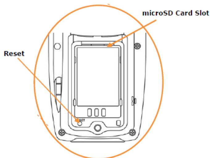
3. Holding the "Left" button, tap the "Reset" button underneath the battery door.
