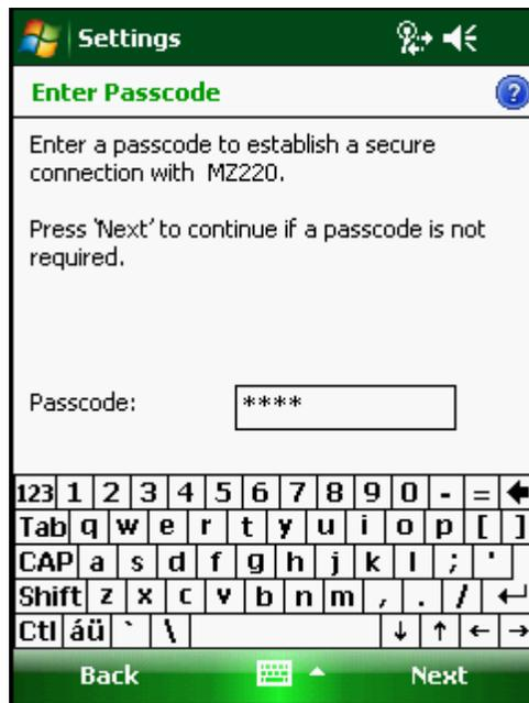
The XM66 will pair with the device. Do not be concerned that its state is Disconnected. At the time this panel appears, it is disconnected.
