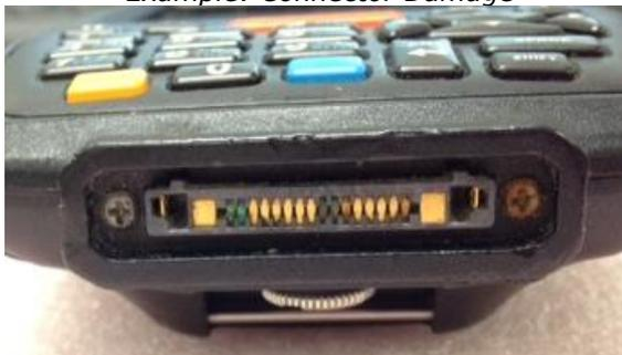
The pins on the cradle base should appear evenly aligned and free of dust, corrosion and/or debris as in the examples below.
