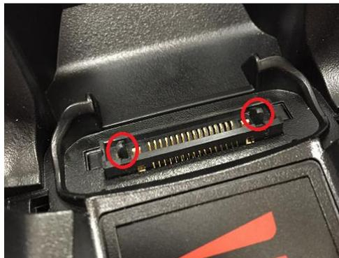
8. Check the cradle housing for proper fit. Janam's single-slot and four-slot cradles accommodate the slight differences in housings with two configurations (noted by the suffix -001 or -002).
